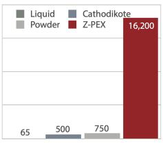
Abrasion Resistance (ASTM D4060)
